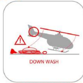
HAZARD - DOWN WASH AND TAIL ROTOR
