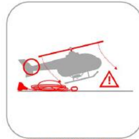
HAZARD - FLAIR LANDING OVER LINES
